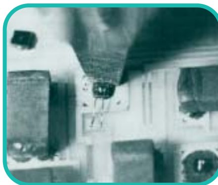
Removing a chip with CE-104
