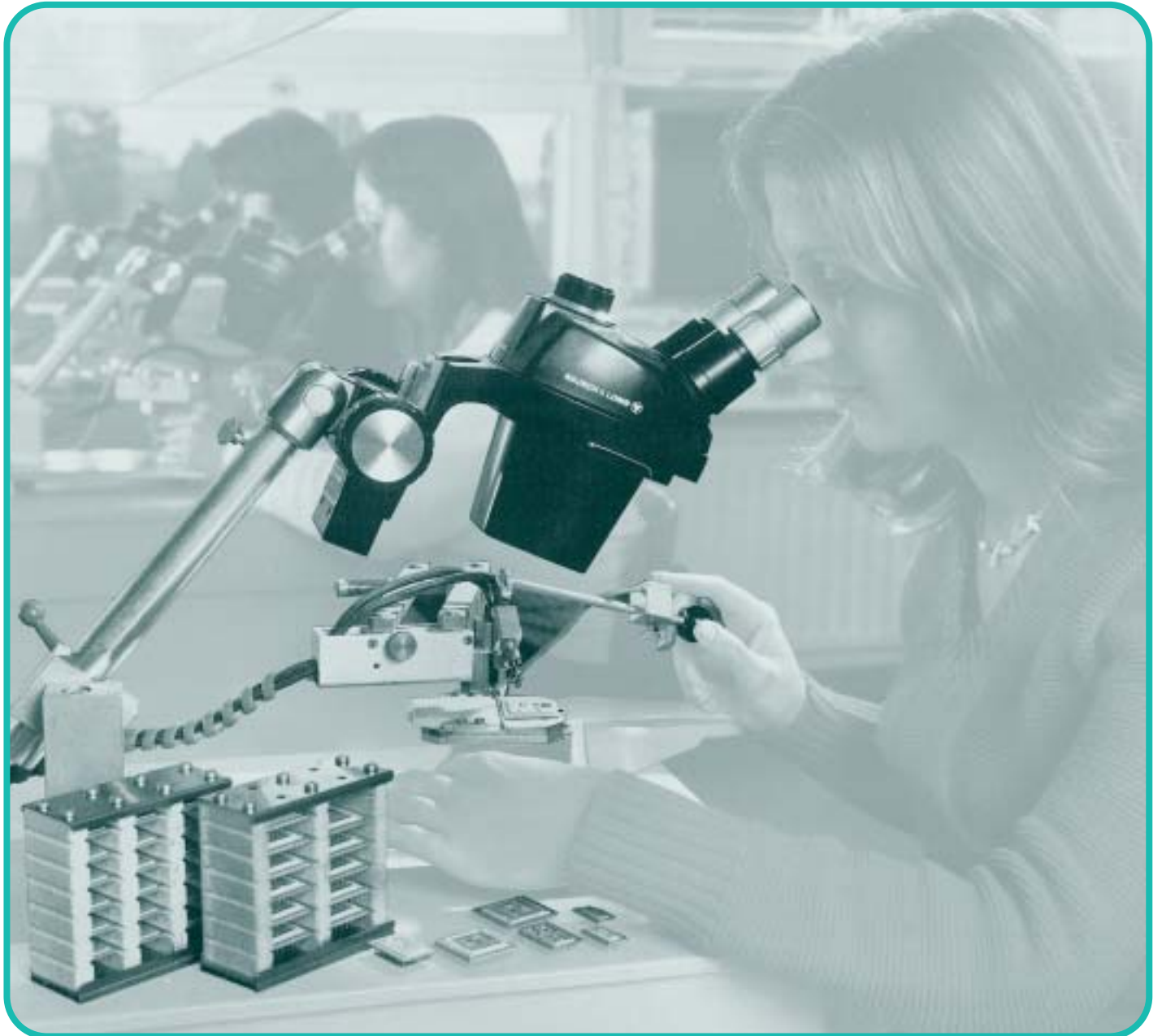
The Micro-Manipulator in use for die mounting
